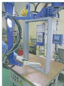
Ex.2 Easy to weld tall workpieces.
