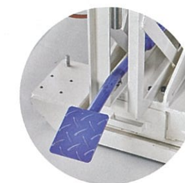
Fix the position by the foot lever first, then pressurization starts.
