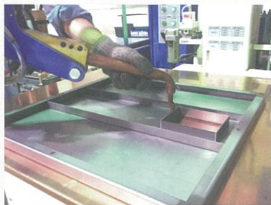
Ex.1 Place a workpiece and move the gun to the welding point.
