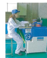
Comfortable welding position.
